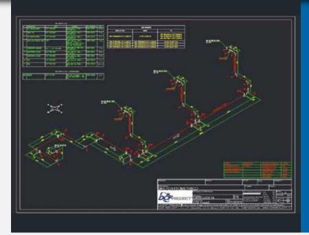
In the isometric design procedure the individual components are represented by symbols, so each manufacturer can read these documents and produce pipes quickly and easily.
